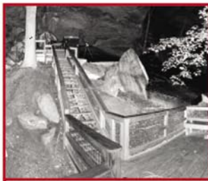
Quantapoint 2D Laser Scan (Not a Picture) Each Point is a Measurement
